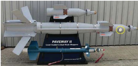
Two GPS antennas (circled in yellow) to provide continuous GPS coverage during weapon flyout through impact.
